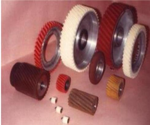
The Castable nature of urethanes – which don't require high pressure like typical rubber and plastic – permits quick, low-cost molds and fast response time in many cases. Top-cast surfaces can be faced off in a secondary operation to achieve precise dimensions. The liquid urethane containing all the mixed ingredients “cures” to a rubbery solid at elevated temperatures. Polyurethane can be made to fit customer requirements with any colour, shape and size with the required shore hardness.
